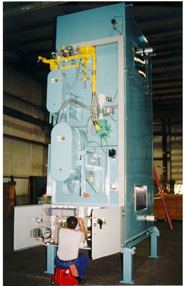
The back of the Sahara V shows the compact modular design of the burner and piping, blower, exhaust system and electrical enclosure.
