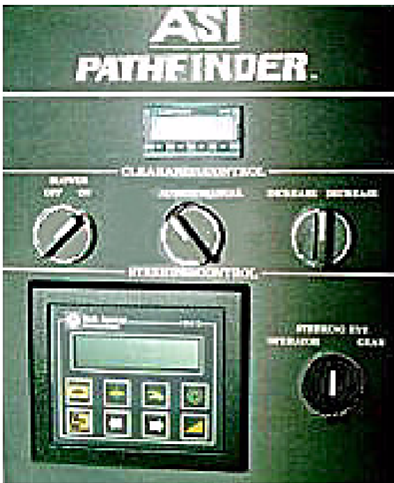
The remote mounted control panel contains all control functions in a simple layout that includes web tension read-out and auto/manual controls for web positioning and air turn clearance.
